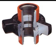
**Figure 602.** 6,000-psi NSCWP unions are available in 1, 1¼, 1½, 2, 3, 4 and 5-inch sizes in standard or sour gas service. These unions feature a resilient nitrile seal ring that helps sealing and protects the steel-to-steel seating of the union. Recommended for manifold and truck-mounting where size and weight are critical. Fig. 602 unions are also available as non-pressure seal unions and in butt-weld Sch. 80, Sch. 160 and XXH, 4" API 8 round threaded ends.
