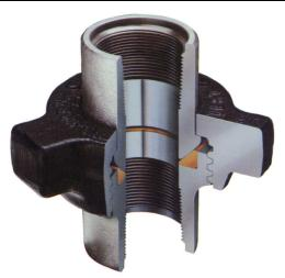
**Figure 600.** 6,000-psi NSCWP unions are available in 1, 1 ¼, 1 ½, 2, and 4–inch sizes. These unions have a bronze seat insert to provide an additional hardness differential across the seats for enhanced sealing.
