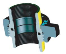
**FIGURE 300.** 2,000-psi NSCWP unions are available in 2-inch line pipe thread size and are also available in 2" and 2½" 8 round EUE thread sizes. These unions feature the effective and dependable "flat-face/o-ring" sealing design. They seal equally well in low or high pressure vapor or liquid service. The "flat-face" design also permits straight away lateral breakouts of short rigid piping sections, without the need to spread the pipe.
