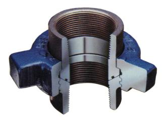
**Figure 206.** 2,000-psi NSCWP unions are available in 1-inch through 10-inch. These unions are fitted with an o-ring in the male sub seating surface for enhanced sealing. Available in butt-weld Schedule 40 and 80. Also available with stainless steel subs.
