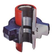
**Figure 1502.** These 15,000-psi NSCWP unions are available in 1, 1½, 2, 3, 4 and 5-inch sizes with a replaceable resilient nitrite seal ring. Alloy steel construction, heavy walls and a rugged design have made these unions popular with the service companies for working pressures up to 15,000-psi. Figure 1502 unions also are available with non-pressure seal threads and in butt-weld Schedule 160 or XXH, 2" or 2½" API 8 round threaded ends or prepped for sour gas service.
