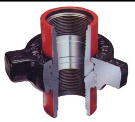
**Figure 400.** These unions are available in 2, 3, 4, 5 and 6-inch 4,000-psi and 12-inch 2,500-psi NSCWP. All three parts are made from steel forgings with heavy walls and a rugged design. They feature ball and cone sealing for easy alignment and dependable seals. Also available in butt-weld Schedule 80 and 3" or 4" API 8 or 10 round threaded ends.
