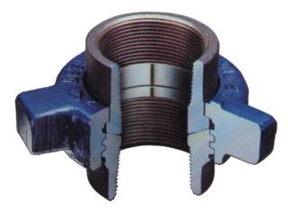
**Figure 200**. 2,000-psi NSCWP unions are available in 1-inch through 10-inch. These unions are compact and popular for low pressure rig piping. They also meet most requirements in the medium pressure ranges for air, water, oil or gas service. Available in butt-weld Schedule 40 and 80. Also available with stainless steel subs.
