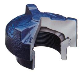
**Figure 207.** 2,000-psi NSCWP unions are available in 3, 4 and 6-inch. These unions are fitted with a nitrile o-ring in a blanking cap for effective closure. With the cap removed, the female sub will make up to hose, pipe or tubing fitted with a Figure 200 or 206 male sub and nut. Recommended for air, water, oil or gas service. Available in butt-weld Schedule 40 and 80.
